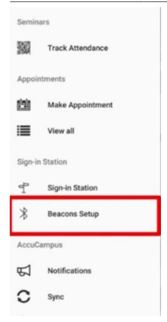
Once Beacon setup has been accessed a list of nearby beacons will appear. Note: If no beacons appear, open the back of the beacon and make sure it is turned on – the blue light should be sustained and not blinking when you press the button.
